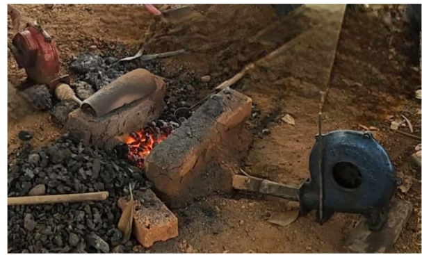
Figure 5: Heating furnace used for forging operations.
